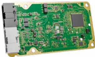
Battery Management Controller (BMC)
